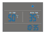
The left side of the temperature display shows the set water temperature. The right side of the temperature
